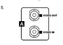
Each monitor has a composite video input (1), with a loop-through output. The video input can be PAL or NTSC, the TLM-433 will automatically detect the video standard.
